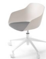
KUSKOOA BI OFFICE CHAIR Five legs swivel with castors, jack for adjustment between 380 mm to 500 mm. Bioplastic shell, seat pad upholstered in fabric, eco leather and leather. Legs available in 2 matt colors: white (RAL 9010) or black (RAL 9004) Seat: H 380/500 mm H 725/845 x L 660 x W 630 mm UNE-EN 16139:2013/Corrected version 2015 (Level L2, extreme use)
