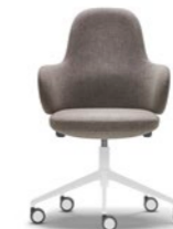
LAN DESK CHAIR 5 legs swivel with castors, white (RAL 9010) or black (RAL 9004) matt finish and jacks for adjustment. Seat height: from 440 to 540 mm. Integrated mechanism for adjusting and lock the backrest angle max 29°. Injected foam fully upholstered for an optimal comfort. H 920/1030 x L 690 x W 652 mm UNE-EN 1335-1:2001/AC:2003 and UNE-EN 1335- 2:2019
