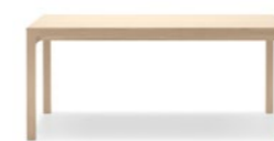
LAIA RECTANGULAR TABLE Solid oak structure. Top in 16mm multi-ply + 4 solid mitre-cut edges in oak veneer (1 mm), 2 faces. Legs in solid oak. Available in square corners or rounded corners. H 760 x L 1400 x W 850 mm H 760 x L 1800 x W 950 mm H 760 x L 2300 x W 1000 mm
