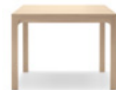
LAIA Legs in solid oak. Top in 16mm multi-ply + 4 solid mitre-cut edges in oak veneer (2 faces). Square corners. H 760 x L 800 x W 800 mm H 760 x L 1300 x W 1300 mm
